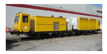
To a clean, safe and reliable network, it is necessary to clean the tracks on a regular basis. For over 50 years, **NEU RAILWAYS** has been supplying the **VAKTRAK®** cleaning train across the world. It is based on the patented design of a combined blowing/suction system. The VAKTRAK® is designed particularly for underground metro network but can also be adapted to railway or LRV networks. Daily use will increase safety and hygiene in the tunnels. It will also protect equipment and rolling
